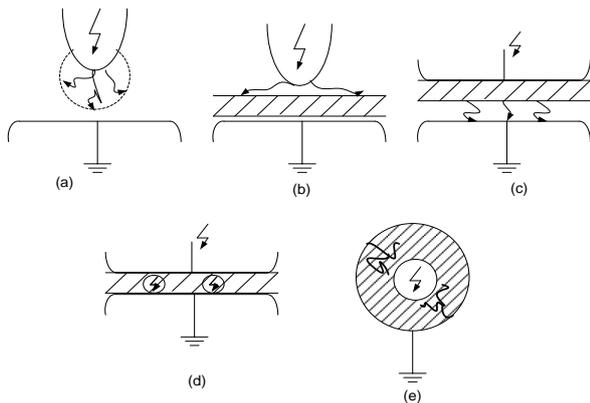
Figure 2: Various discharges a) Corona discharge b) Surface discharge d) Partial discharge
