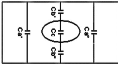
Figure3: Typical three-capacitance equivalent circuit or 'abc' model
